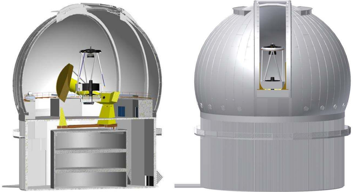
Figure 2: Existing CFHT Enclosure and Telescope
